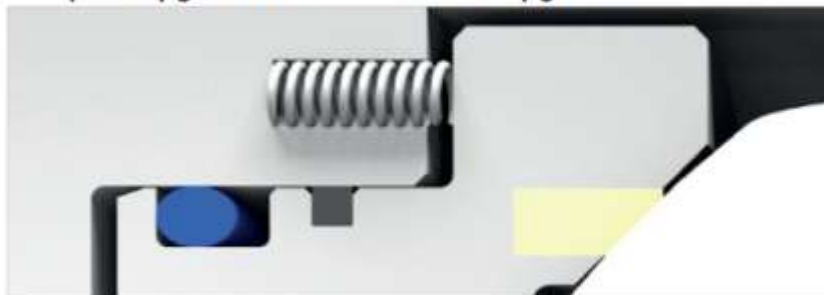
PMSS Primary Metal Soft Seal Soft primary gasket and metal secondary gasket
