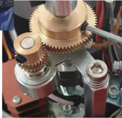
Change the potentiometer value by altering the gear
